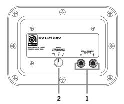
1/4" TS Full Range Input / Output Jacks: The jackplate features two 1/4" jacks wired in parallel, allowing easy daisy-chaining from one speaker to another. Each of the jacks may be used as an input or a through connection.
